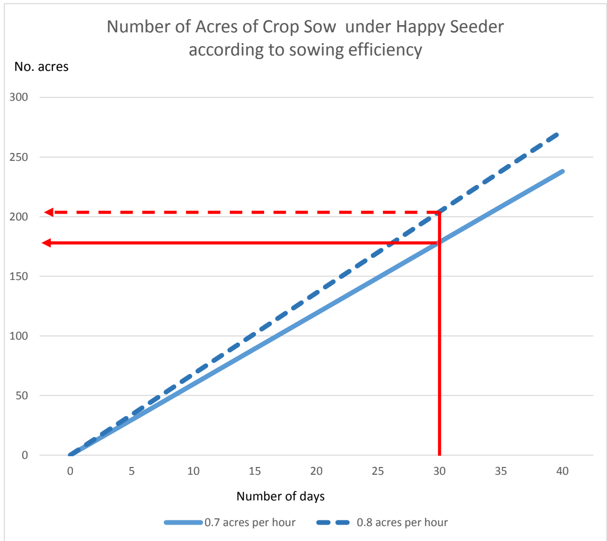
Figure 56: Number of days that the HS will need to operate to sow a range of different crop areas
