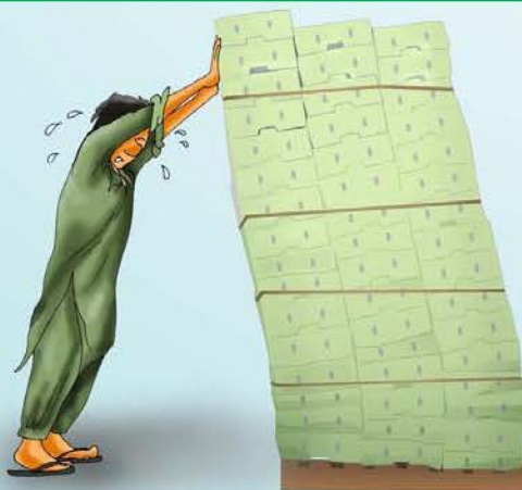
Weak cartons collapse leading to poor alignment in pallets
