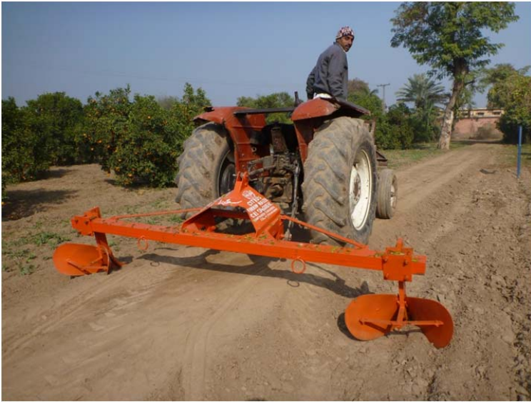
Figure 4: A tractor drawn ridger implement to make furrows
