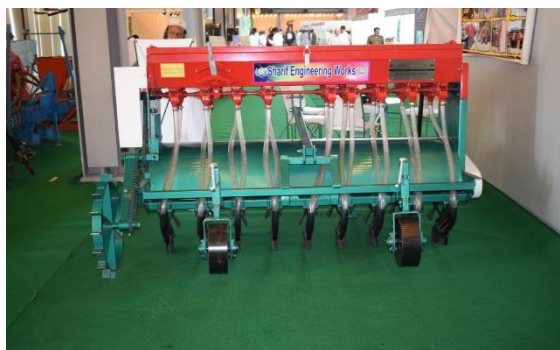
ZTHS with wheels manufactured by Sharif Engineering, Faisalabad
