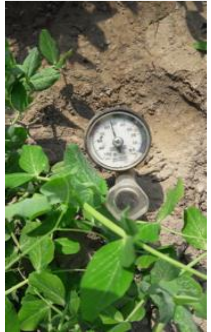
Tensiometer for assessment of soil moisture.
