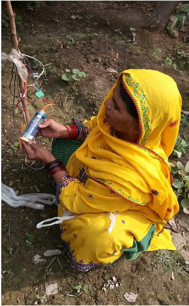
Chameleon reader shows soil moisture at four depths.
