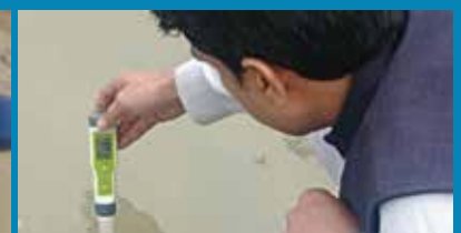
Measuring salinity of water using electrical conductivity (EC)
