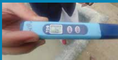
Measuring salinity of water using total dissolved solids (TDS)
